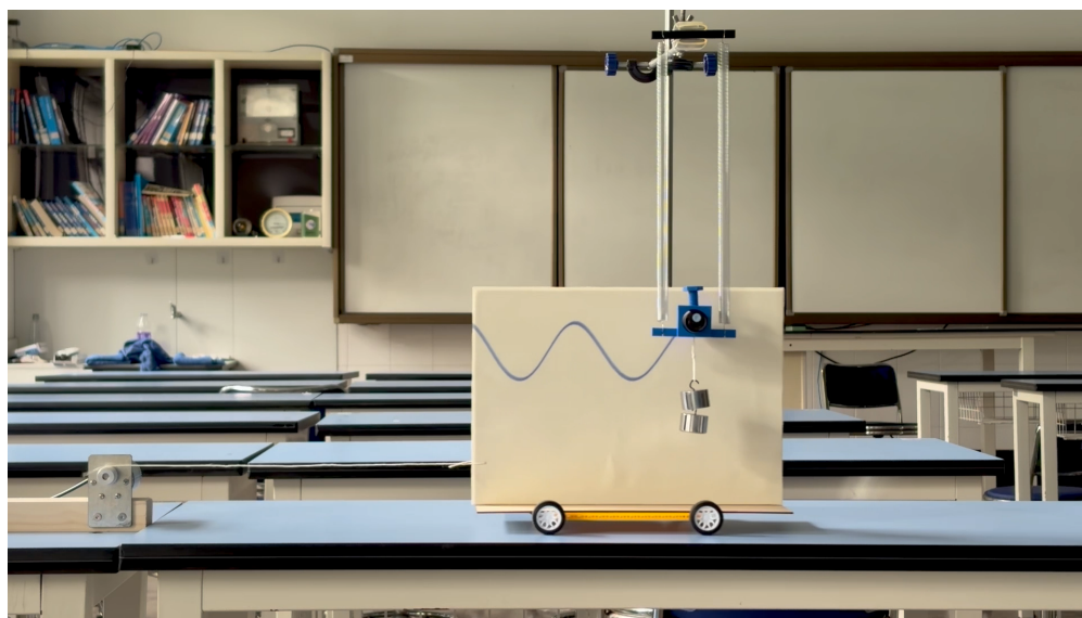
Figure 1: The laser–phosphor recorder during a run. A violet laser pointer below a parallel-spring oscillator writes a glowing sinusoid on the phosphorescent foil mounted on a cart towed along the bench at a few centimeters per second.
